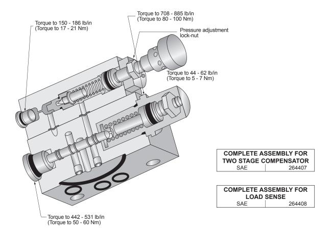
NOTE: Quanity of 3, M6 socket head cap screw, not shown. Mounts 2nd stage to 1st stage compensator. Torque to 133 - 177 lb/in (15 - 20 Nm)
