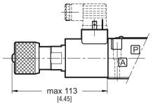
M - Push and twist manual override (only for DC solenoid valve) Code: M3401150026
