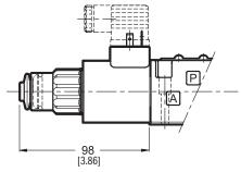
Knob manual override, turning (only for DC solenoid valve)
