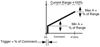
This module has a software adjustable "dead zone" near zero, termed TRIGGER. With a command in this near zero area, neither solenoid will be energized. Trigger is intended to keep small noise signals on the analog command from causing either solenoid to be energized.
