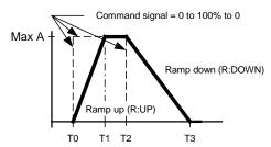
All ramp rates are set via software. All ramps are specified in milliseconds, and are actually "time to ramp for a 0 to 100% signal change." For example, a value of 2000 will give a ramp time of 2 seconds for a 0 to 100% step command. The ramp time will be 1 second for a step command of 0 to 50%.
