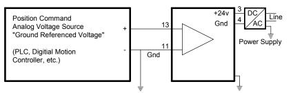
An external position command voltage source must be referenced to ground for proper operation.
