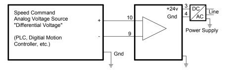
A ground referenced speed command must be referenced to the CEM-MS ground.
