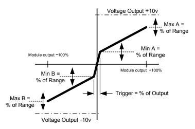
TRIGGER and MIN can be used together to optimize valve performance near zero.
