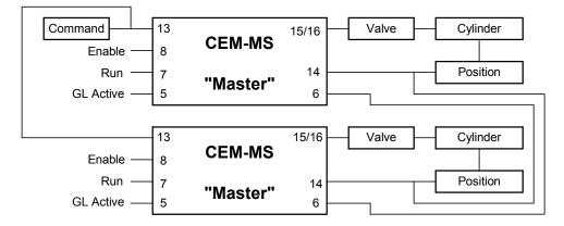
Up to four axis may be synchronized in the "Master – Slave" mode.
