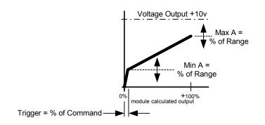
Valid values for MAX:A and MAX:B are 5000 to 10000. Units are 0.01%. Default is 10000. Valid values for MIN:A and MIN:B are 0 to 5000. Units are 0.01%. Default is 0.
