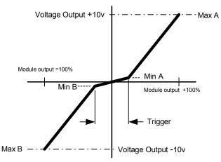
When setting the OUTPUT parameter to UNIPOLAR, the adjustment of MIN:A and TRIGGER are usually less important then when in BIPOLAR mode. But similar control concepts apply.
