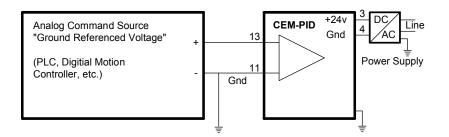
Pin 12 is a regulated 10vdc output pin that may be used as a reference voltage for generating command signals. It is limited to 10mA output. It is internally referenced to module ground (pins 4 and 11).
