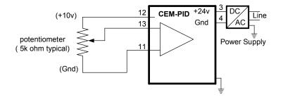
An external voltage source must be referenced to ground for proper operation.
