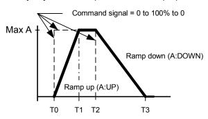
Ramp rates are set via software. All ramps are specified in milliseconds, and are actually "time to ramp for a 0 to 100% signal change." For example, a value of 2000 will give a ramp time of 2 seconds for a 0 to 100% step command. The ramp time will be 1 second for a step command of 0 to 50%.
