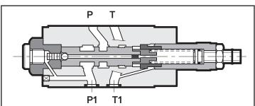
The P05MSV-SP is a direct operated spool type sequence valve and is used to control two or more actuators in succession. The mounting surface conforms to NFPA D05/ISO 4401-05 standards.
