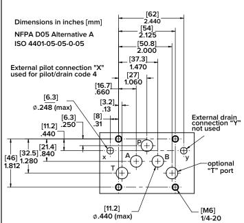
The valve with internal pilot can be installed both on NFPA D05 (ISO 4401-05-04-0-05) and NFPA D05 Alt A (ISO 4401-05-05-0-05) mounting interface.
