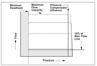
Flow Versus Pressure Characteristic Curve.
