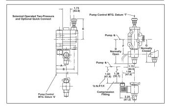
Using the hydraulic code on the pump name plate, determine if the solenoid id normally open or closed. An example hydraulic code of a vented control is: PVX-60B25-XX-XX-**29**24-A. In this example, the **29** identifies the pump as a vented compensator with a **normally open** solenoid. If the code had a **30** in this place, the solenoid is **normally closed**.
