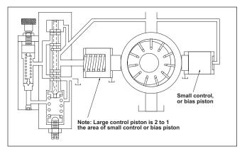
To set-up a two-stage compensator, follow the instructions given in the previous section *"Proper Setting of the Thrust Screw"*. Once this is done, adjust and lock the compensator knob at the maximum compensating pressure of your system.
