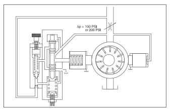
Load Sense Flow Compensator (LSFC).
