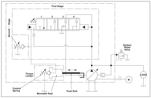
Torque Limiter Schematic.
