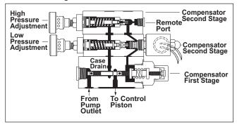
stages will have control of the pump. Soleniod Two-Pressure Compensator.
