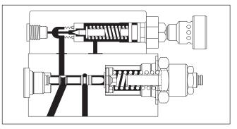
Two-Stage Compensator Cut-Away View.
