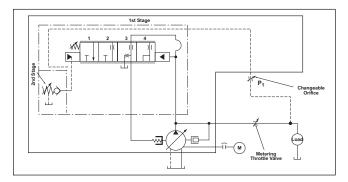
Load Sensing Flow Compensator Schematic.
