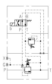
Pressure Relief, 2 pressure, normally low pressure, energize for high pressure
