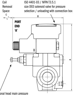
Hexagonal head main pressure adjustment screw: 13 mm [1/2] wrench Clockwise rotation to increase pressure
