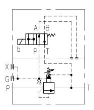
Pressure Relief, normally high pressure, energize to unload
