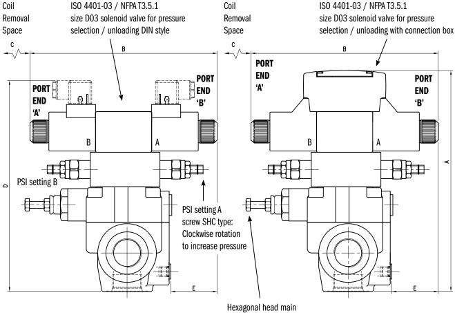
Hexagonal head main pressure adjustment screw: 13 mm [1/2] wrench Clockwise rotation to increase pressure Dimensions in mm [IN]
