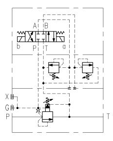
Pressure Relief, 3 pressure, normally highest pressure, energize A solenoid for pressure setting A energize B solenoid for pressure setting B
