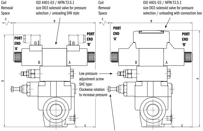
Hexagonal head main pressure adjustment screw: 13 mm [1/2] wrench Clockwise rotation to increase pressure
