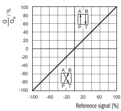
Typical flow rate curves at constant  $\Delta p = 70$  bar P-T according to the reference signal. NOTE: with positive reference signal connected to pin D the valve regulates P - A / B - T.
