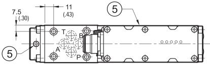
Valve Bolts: 4 SHC screws 10-24 NC x 1.25" ASTM A574 (BD03-125) Torque: 4-6 lb.-ft. (5.4 - 8 Nm)
