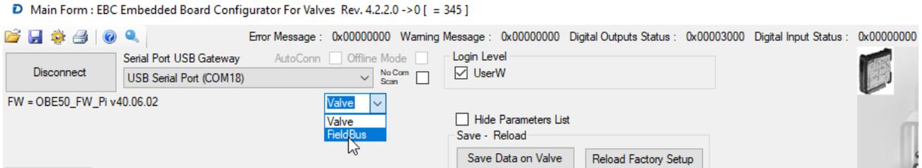
Select Disconnect and Connect, the connection to Fieldbus is displayed:
