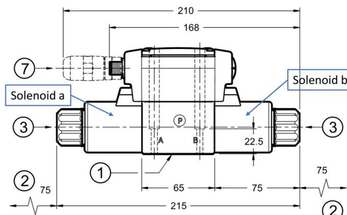
For 1-solenoid valves, solenoid "a" refer to the only solenoid available, independently if valve is type SA or SB. For 2-solenoids valve, the hydraulic function is according to the Spool Type, check catalogue for further details:
