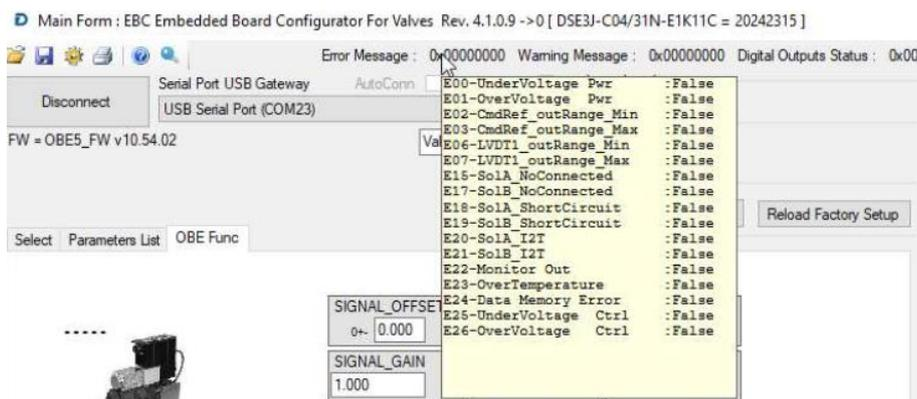
For E1 valves with output monitor function on pin F, in case of error detected, the output current value is set to a value lower than 3 mA (this is valid if valve is not connected with LinPC).
