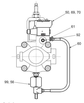
Code 8Rate Control Valve for Dual PressureCode 9Rate Control Valve for Dual Volume
