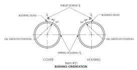
3. After the bushings are in place, check to see that the rotorshaft will fit into the bushings and provide a smooth turning fit. If the shaft turns hard, the bushings should be removed and the bore checked closely for nicks or burrs before pressing in the new bushings.
