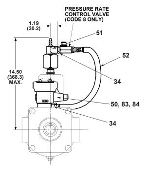
Code 2400 Dual Volume Control Without Integral Valve (32A, 42A, and 50B Only)
