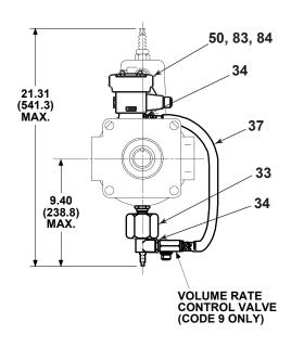
Code 2500 Dual Pressure/Volume Control Without Integral Valve (32A, 42A, and 50B Only)
