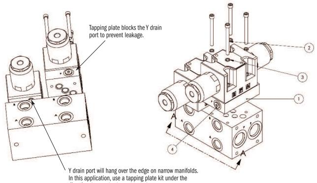
In this application, use a tapping plate kit under the directional control valve to block the port. Use a manifold with a D05 alt A mounting pattern for applications where the drain port is required.
