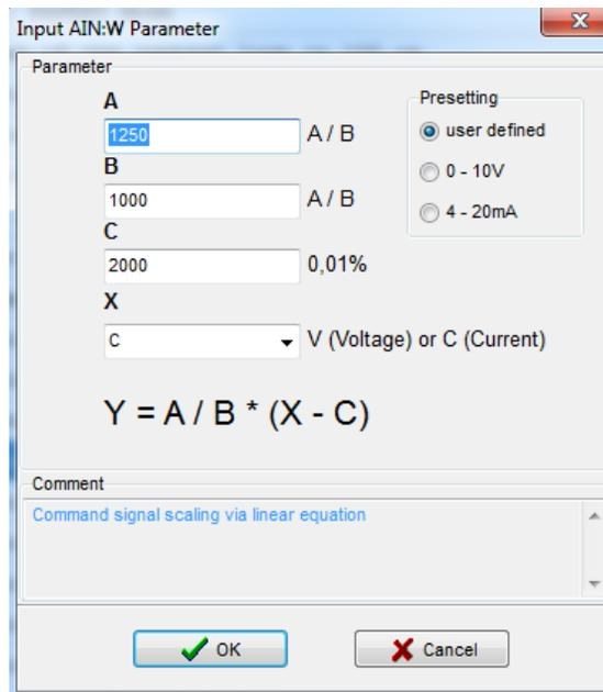
**AINMODE - Analogue input scaling parameters**
