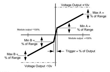
TRIGGER and MIN can be used together to optimize valve performance near zero.
