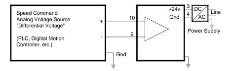
A ground referenced speed command must be referenced to the CEM-SA ground.
