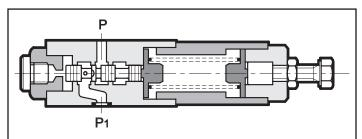
The P03MSV-SP valve is a direct operated sequence valve of the spool type and is used to control two or more actuators in succession.
