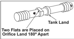
increases and the balance of forces determines the spool position. The spring cavity of the compensator is drained to the tank to prevent any pressure buildup from leakage, which would add to the spring force and change the compensator setting.
