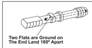
If there is a pressure spike in the system above the compensator setting, the spool will momentarily move to the over travel position in an effort to destroke the pump. Only in position #2 is it a true compensating condition. Do not be confused with the term "deadhead", it means the same thing as compensating.
