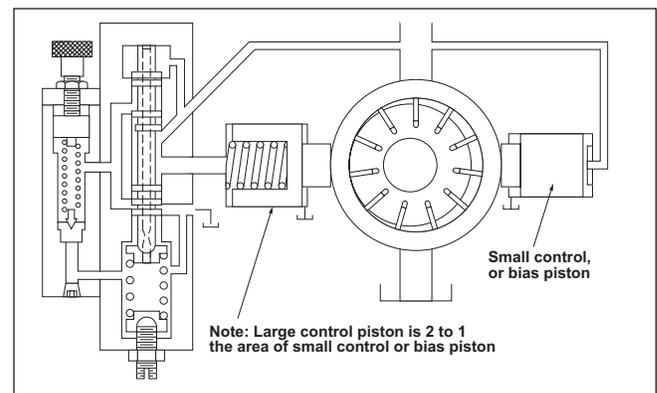
To set-up a two-stage compensator, follow the instructions given in the previous section "Proper Setting of the Thrust Screw". Once this is done, adjust and lock the compensator knob at the maximum compensating pressure of your system.
