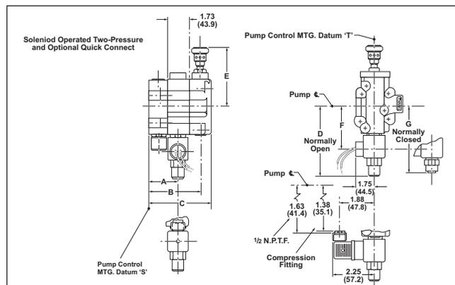
Using the hydraulic code on the pump name plate, determine if the solenoid is normally open or closed. An example hydraulic code of a vented control is: PVX-60B25-XX-XX-**29**24-A. In this example, the **29** identifies the pump as a vented compensator with a **normally open** solenoid. If the code had a **30** in this place, the solenoid is **normally closed**.
