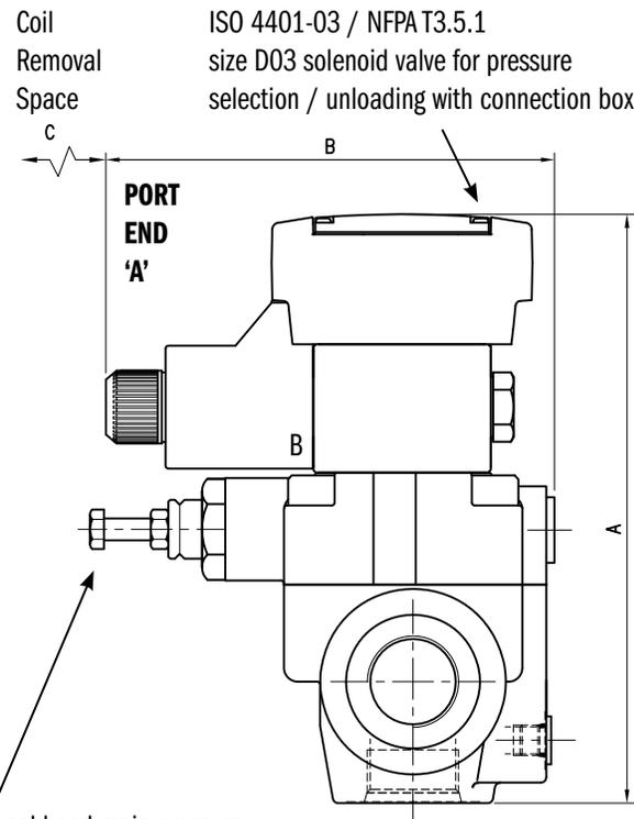
Hexagonal head main pressure adjustment screw:
