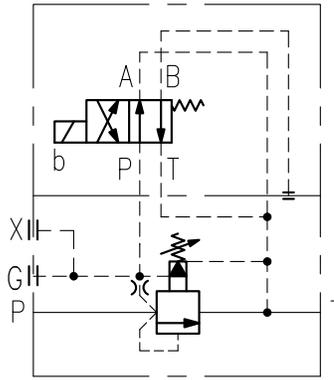
Pressure Relief, normally unloading, energize to high pressure
