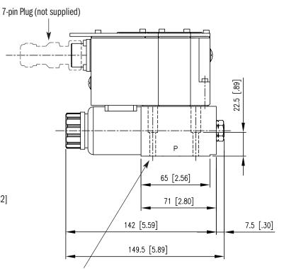
Mounting surface with sealing rings: 4 pcs. AS568-012 90 Shore A Ports A and B are blind holes with O-Ring seats.
