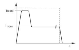
**ECG** This version enables hydraulic actuators to perform a smooth start and stop by setting times values (200 - 600 ms) for ramp up and ramp down. See available spools in the catalog Variables should be used in IO-Link are ONOFF\_TON and OFFON\_TOFF.
