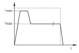
**ECF** This version allows a fast switching, over boosting the 12 V solenoid just for the time needed to energize it. Then, the voltage will be lowered at the nominal value. The de-energizing is fast, around 10 ms. At over boosting time, the power-supply unit must be able to provide a 6 A current with 24 V supply voltage.
