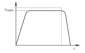
**ECL** This version allows to feed the solenoid at the nominal current value for a time sufficient to guarantee the complete valve energizing (200 ms). The current is therefore automatically reduced at holding (approx 60%). The IO-Link mode that correspond to these versions is ECO, it is possible to set the hold current percentage of the nominal current by parameter ONOFF\_ECO, and set the power on time by parameter ONOFF\_TECO
