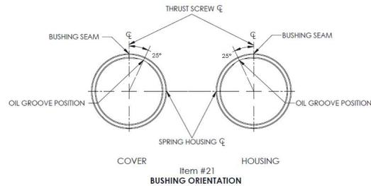
3. After the bushings are in place, check to see that the rotorshaft will fit into the bushings and provide a smooth turning fit. If the shaft turns hard, the bushings should be removed and the bore checked closely for nicks or burrs before pressing in the new bushings.
