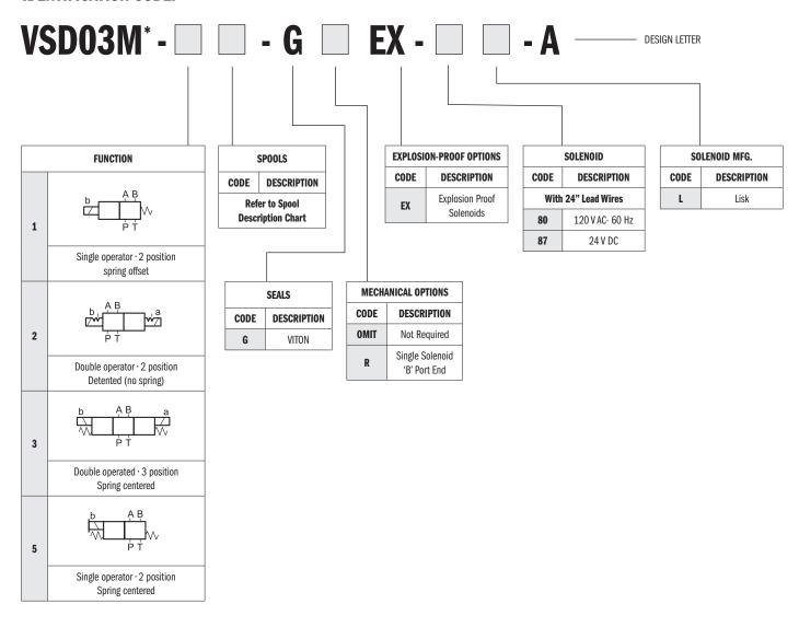
Note: The complete VSD03M valve assembly is not CSA or UL certified. However, the Lisk solenoid valves are certified. Rise block included.
