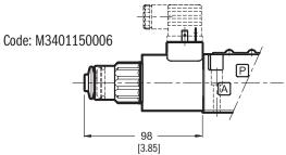
**CPK Push manual override with mechanical retention**
